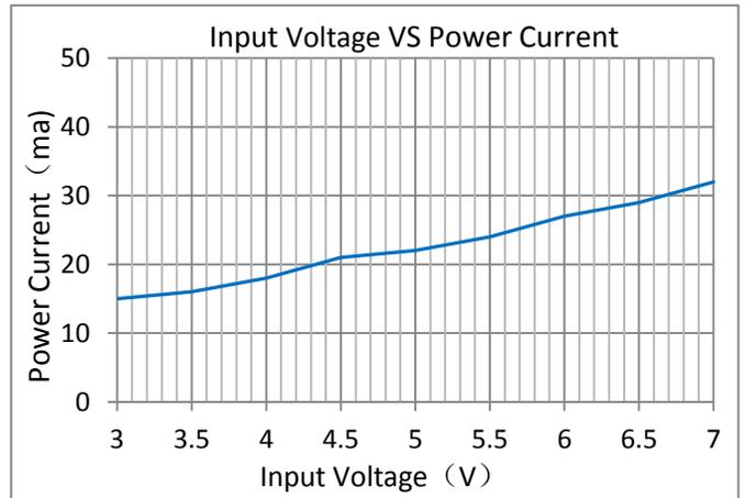
图6: Power Crrnt VS. Supply Voltage
